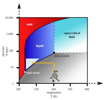
Figure 2 Phase diagram of pure CO<sub>2</sub> with ranges for CO<sub>2</sub> capture and shipping transport indicated. Figure modified from [24].
