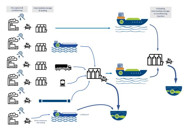
Figure 1 Simplified value chain alternatives for CCS. Note: Pumping not shown. A list of icons is in Table 2.
