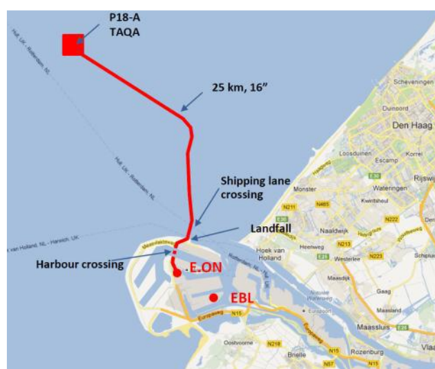
Figure 4. Location of the ROAD project and its CO 2 transport lane at reclaimed land at the Rotterdam harbour
