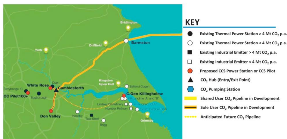
Figure 3. Don Valley project location in the Yorkshire and Humber region of the UK, with the originally planned transportations system comprising of a 68 kilometre onshore. At Barmston the onshore pipeline is connected to an offshore pipeline
